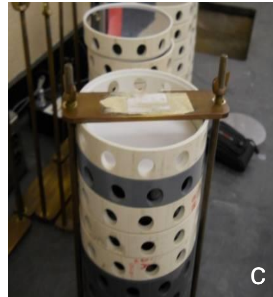
a) TAPPI Handsheet forming , b) Handsheet pressing, c) Handsheet drying
