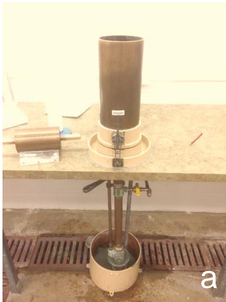
a) TAPPI Handsheet forming , b) Handsheet pressing, c) Handsheet drying
