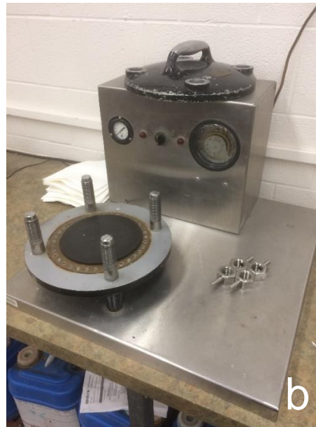
a) TAPPI Handsheet forming , b) Handsheet pressing, c) Handsheet drying
