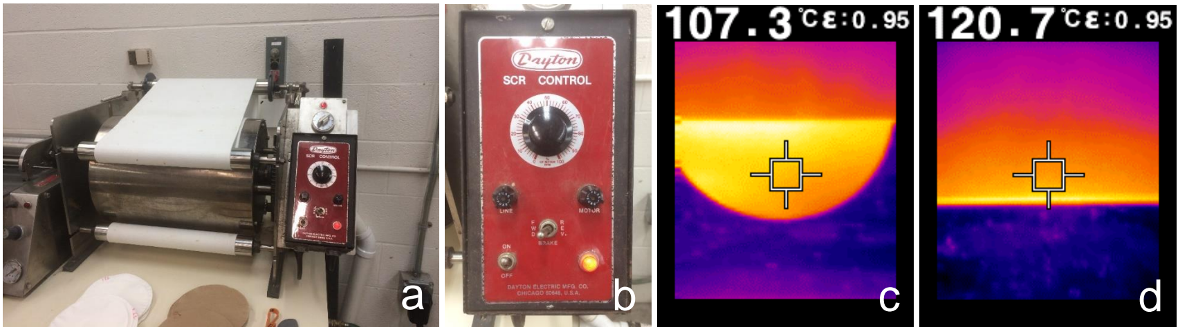
a) Dayton photo dryer, b) Control unit, c) Handsheet drying , d) Drying felt/cylinder
