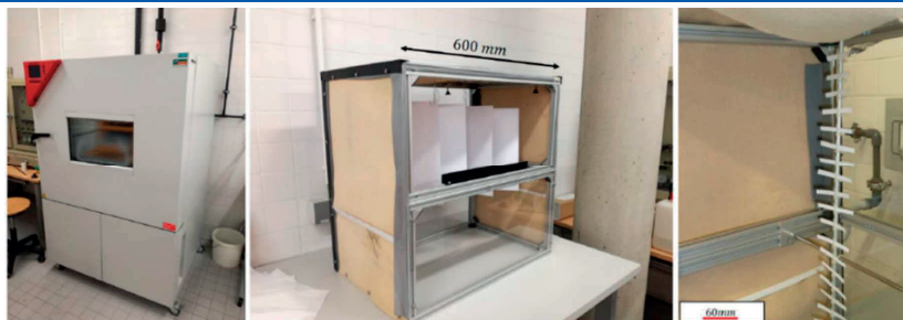
Fig. 5. Laboratory equipment for climate experiments. Climate chamber (left), self-built case for probe protection (middle) with sample holder where the 6 \times 6 mm specimens were placed (right)
